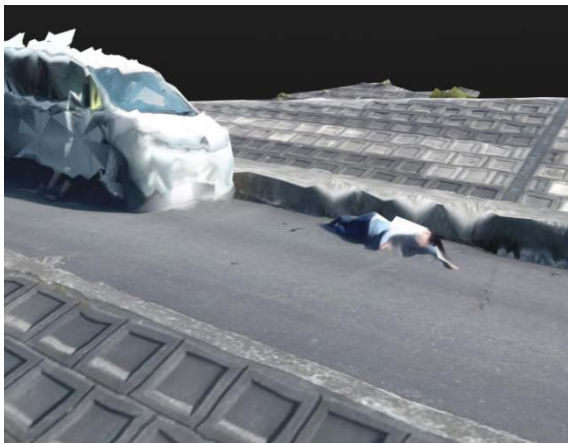
Fig. 4: 3D model by 90%lap.
