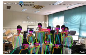
Fig. 11: An example of posture detecting by the Open Pose
